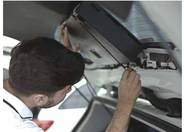
Three boxes were mounted into the back and into the side windows of each measuring car in order to support twelve smartphones per car.
