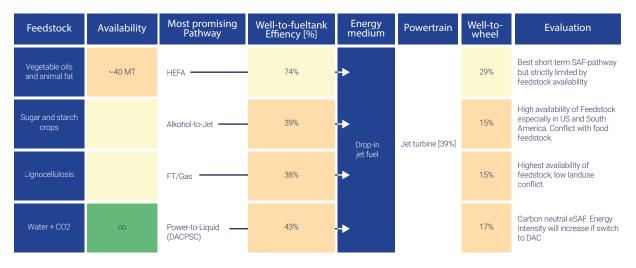
Figure 7: Efficiency of different SAF pathways is comparable.
