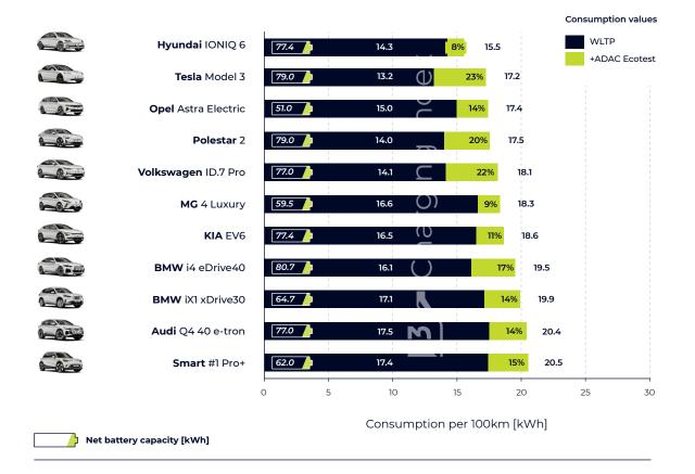
Premium class vehicles are generally equipped with smaller batteries than luxury class models, which can result in a lower battery weight and therefore lower consumption. The range here extends from at least 51kWh in the Opel Astra Electric Sports Tourer GS to just under 81kWh in the BMW i4 eDrive40. The Hyundai IONIQ 6 is particularly noteworthy, achieving an extremely low
