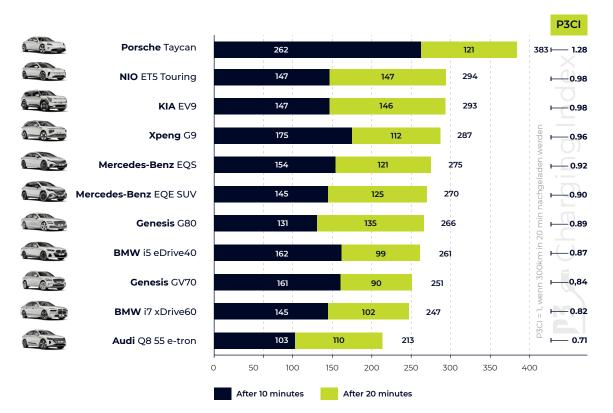
**The Porsche Taycan is in first place** in the luxury class of the P3 Charging Index and can recharge 262km of range in 10 minutes. In total, the saloon recharges 383km in 20 minutes. The Taycan thus impressively demonstrates the advantages that high charging performance in combination with low consumption can bring.
