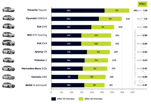
For the first time, the TOP 3 of the P3 Charging Index in the overall ranking all charge more than 300km real range in 20 minutes and thus have a P3CI greater than 1.0.
