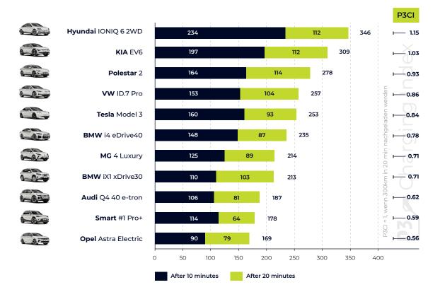
**The Hyundai IONIQ 6** is capable of recharging a range of 234km in just 10 minutes, with a total range of 346km achievable within 20 minutes, making it the winner of the premium class category of the P3 Charging Index. This demonstrates how a high charging capacity in conjunction with relatively low consumption can markedly extend the recharged range in 20 minutes.
